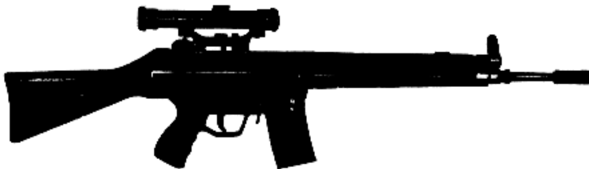
Fig. 7: HK33ZF from the right Rifle HK33 with telescopic sight
